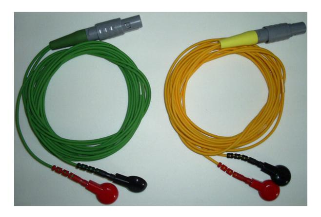
Mind that when connecting the two plugs that they are coded with both colors and different guide grooves. So it is only possible to insert the yellow plug into the yellow socket and the green plug into the green socket. The plugs must be inducted so far so they catch noticeable. To remove the connection pull back the shell of the plug, only then the lock will disconnect and the plug can be pulled out. The negative pole of every wire is marked with a black point on the electrode push button.
