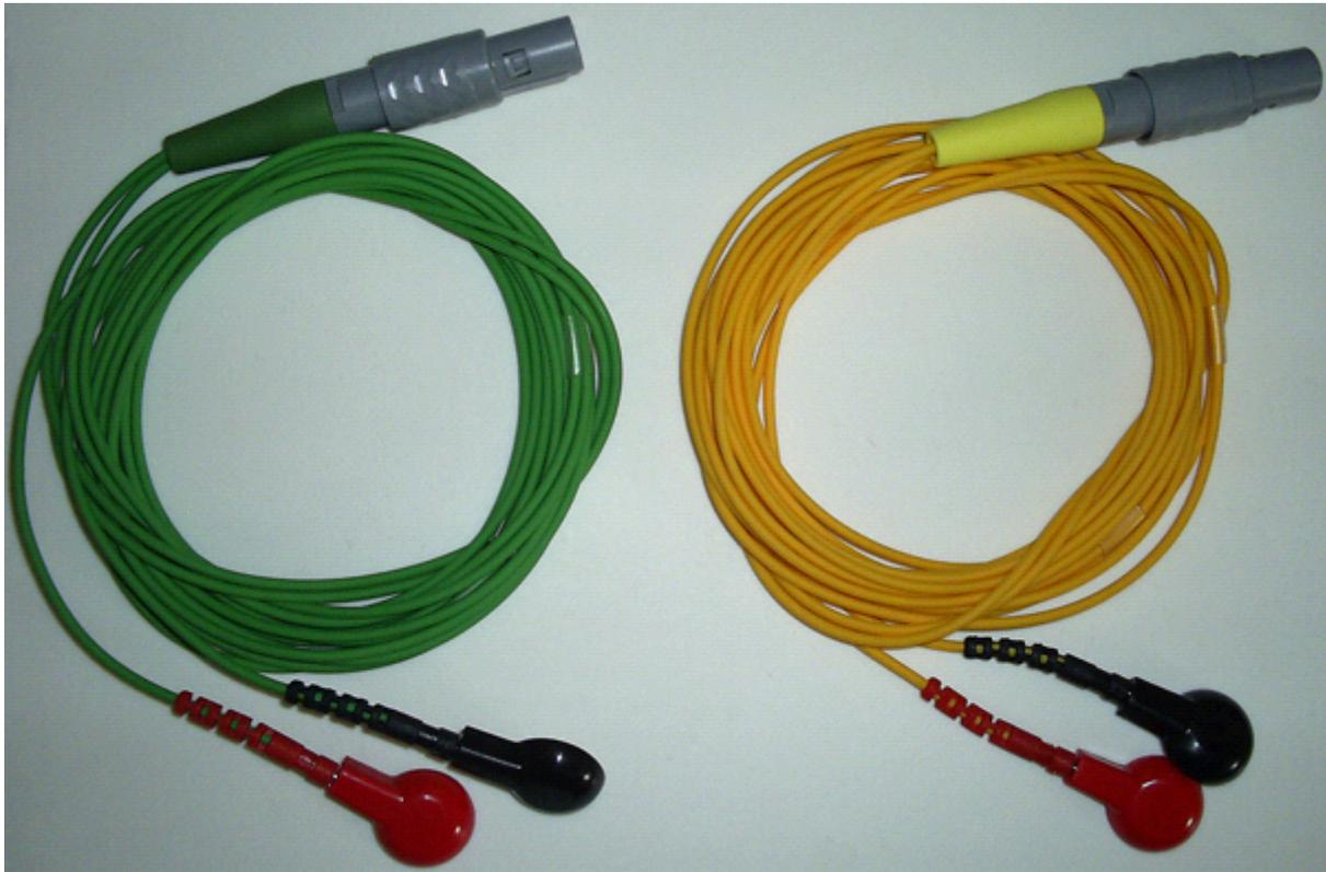
Mind that when connecting the two plugs that they are coded with both colors and different guide grooves.
