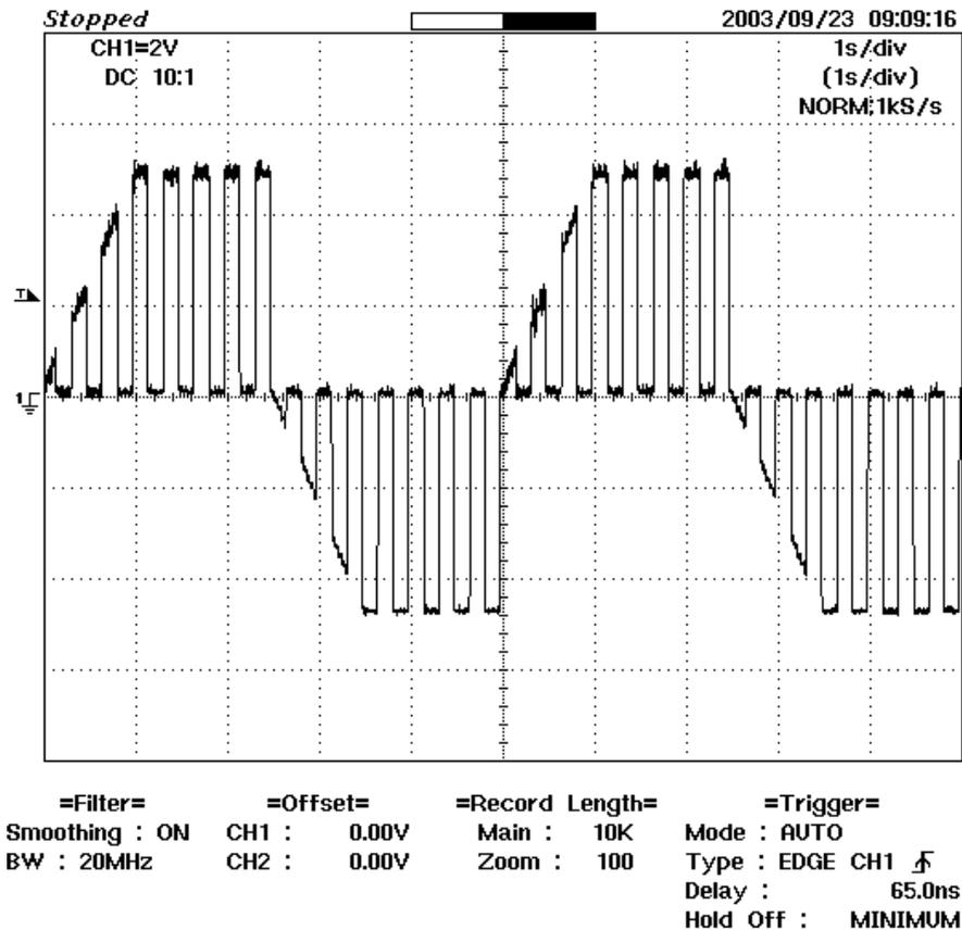
The tension at a load of 10 Kilo ohms with the following parameters was measured:
